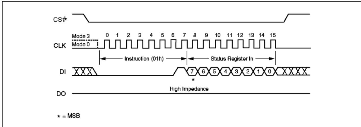
Figure 14. Write Status Register Instruction Sequence Diagram
