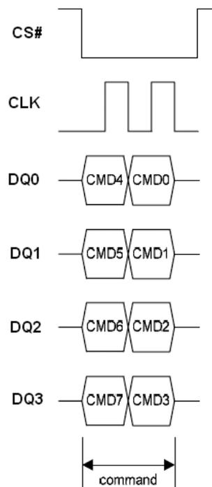
Figure 10.1 Write Enable/Disable Instruction Sequence in QPI Mode
