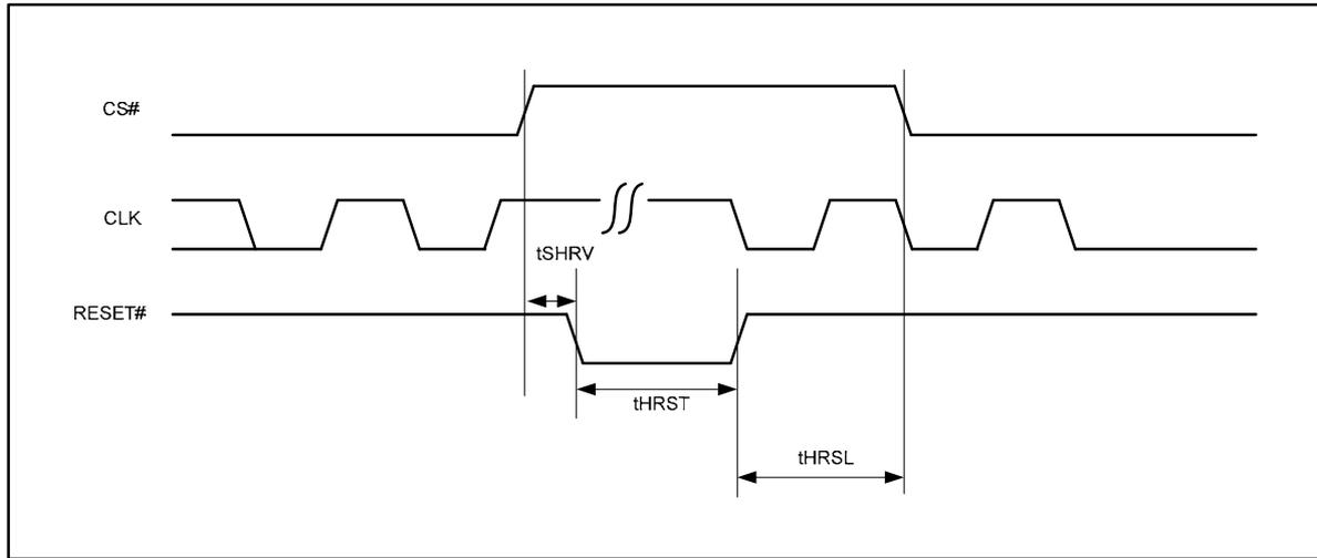
Figure 33. Reset Timing
