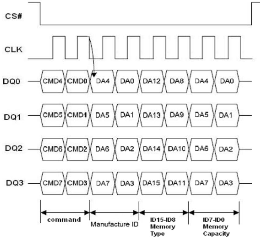
Figure 36.1. Read Identification (RDID) in QPI Mode
