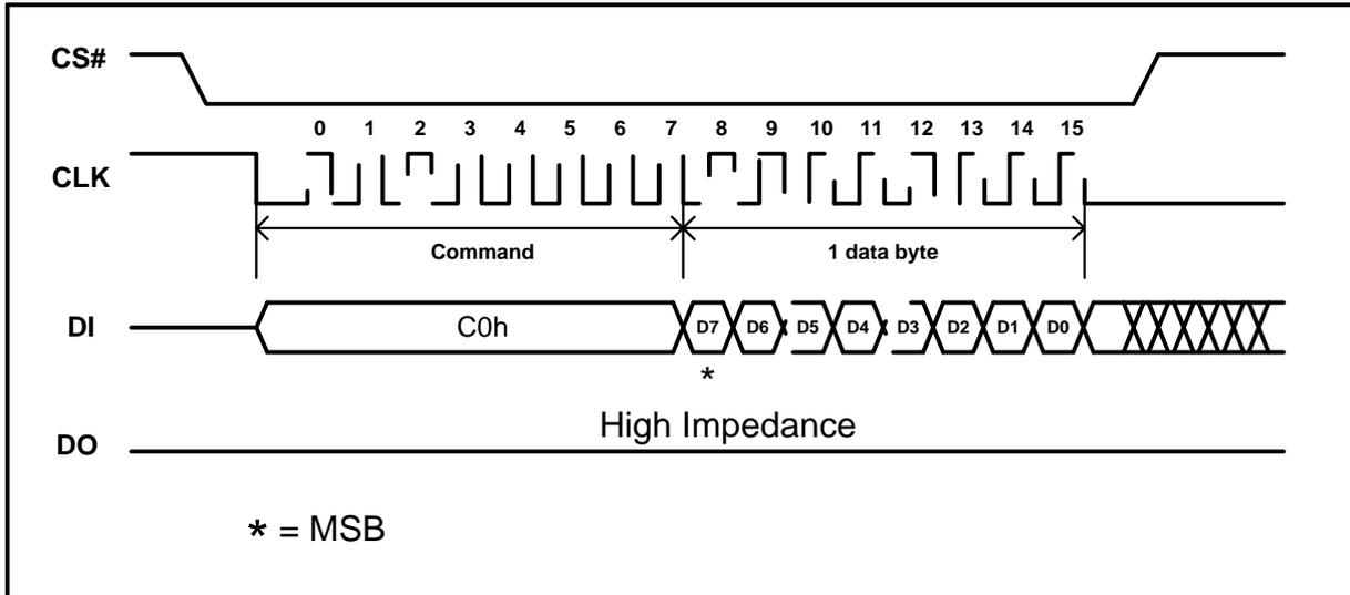
Figure 22. Write Status Register 3 Instruction Sequence Diagram
