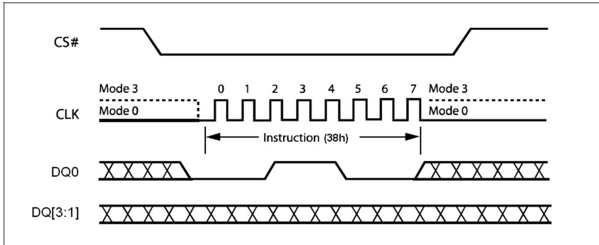
Figure 7. Enable Quad Peripheral Interface mode Sequence Diagram
