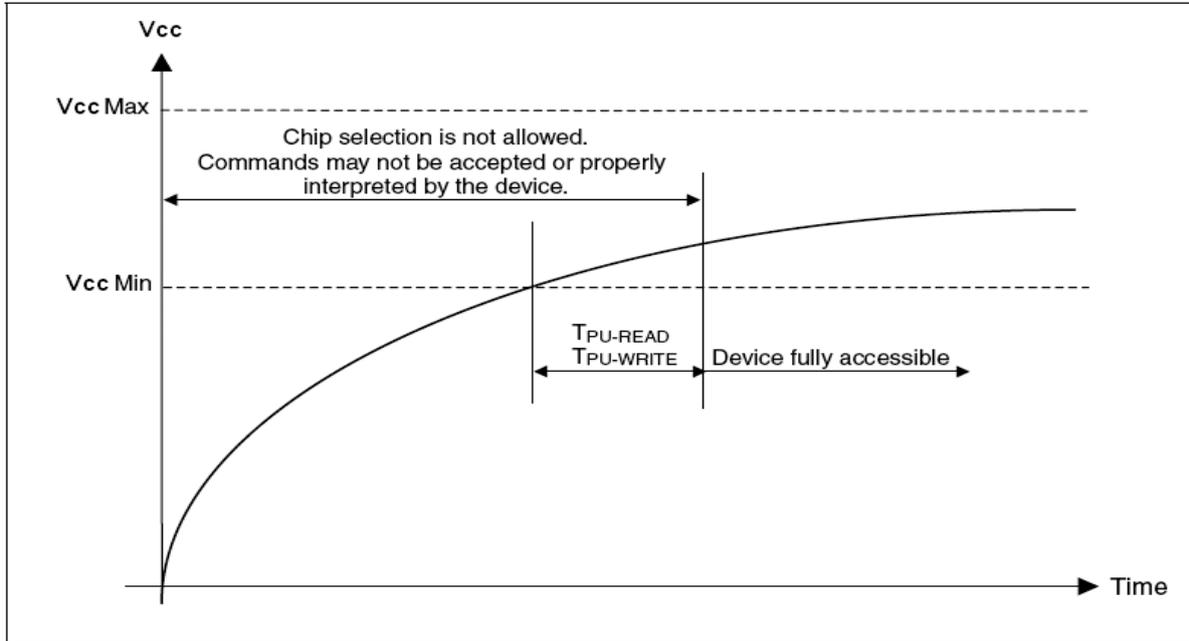
Figure 28. Power-up Timing
