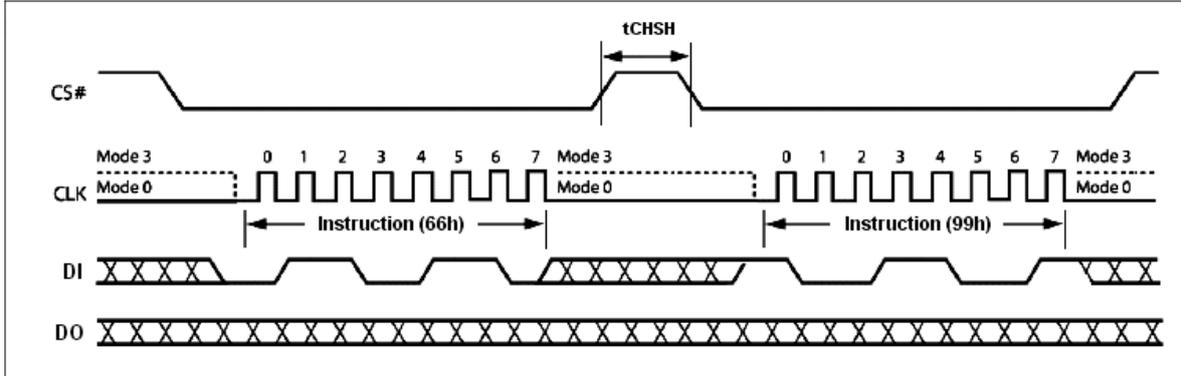
Figure 6. Reset-Enable and Reset Sequence Diagram
