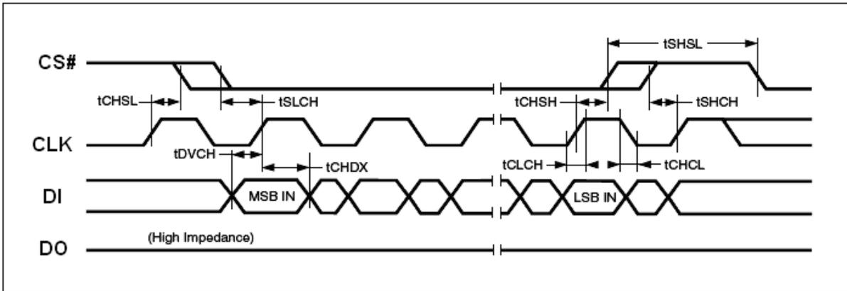
Figure 31. Input Timing
