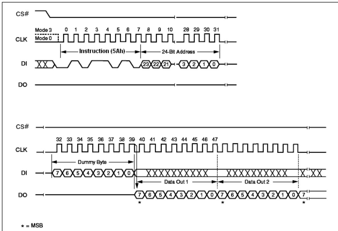
Figure 38. Read SFDP Mode Instruction Sequence Diagram
