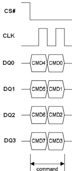
Figure 37.1 Enter OTP Mode Sequence in QPI Mode
