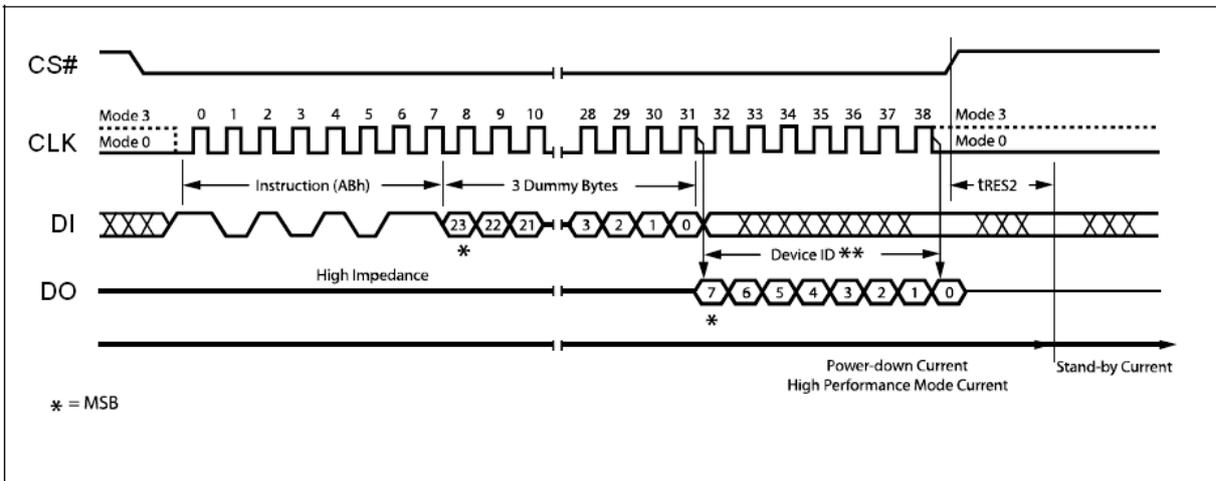
Figure 34. Release Power-down / Device ID Instruction Sequence Diagram
