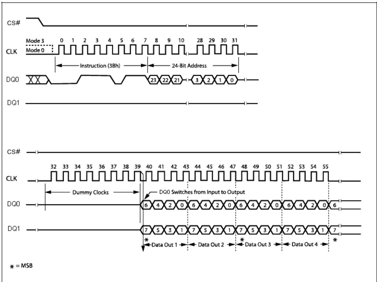
Figure 17. Dual Output Fast Read Instruction Sequence Diagram
