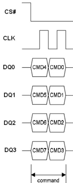
Figure 31.1 Chip Erase Sequence in QPI Mode
